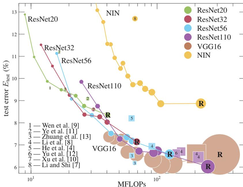
Figure 2: Error-compression space of test error (Y axis), inference FLOPs (X axis) and number of parameters (ball size for each net), on CIFAR10 models (different color for each model family). Results of our algorithm span a curve, shown as connected circles; **R** — reference model.
