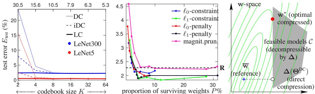
Figure 1: *Left*: error-compression curves for LeNet neural nets using quantization. *Middle*: same but using pruning. *Right*: illustration of the idea of model compression by constrained optimization.
